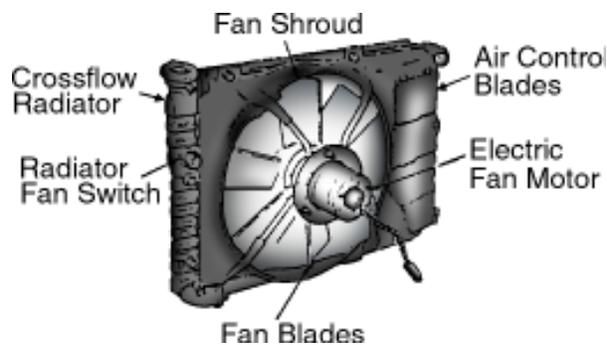
**CAUTION:** Electric fans are wired “hot” from the electrical system. This means electric fans can come on even when the ignition switch is off. Never work on or near an electric fan unless the battery ground has been disconnected. If the electric fan should come on during a service procedure, serious injury could occur.
