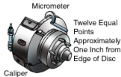
2. If the rotor is parallel, proceed to section C below and measure the rotor runout. If the rotor is not parallel, calculate the rotor's thickness if it is machined to the smallest micrometer measurement.
