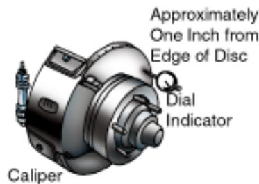
6. To remove runout, reduce the rotor thickness by one half of the runout measurement. For example, if the runout is .006 in, then reduce the rotor thickness by .003 in.
