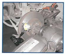
Measuring runout before and after the rotor has been machined can save a comeback.
