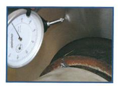
Measuring the runout in the rotor and hub is critical to performing a pulsation free brake job.
